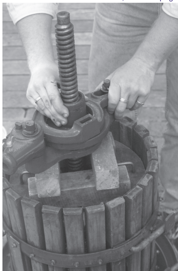
Placing the wood blocks and press head into the press before pressing the grapes.
